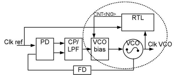
Fig. 8. PVT detection and compensation in a PLL
