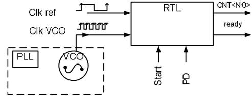
Fig.5. Blok diagram of the PVT sensing circuit
