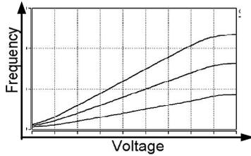
Fig.3. VCO frequency V.S. control voltage for different process corners
