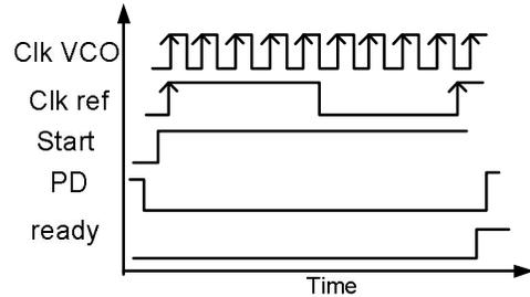
Fig.6. Simplified timing diagram
