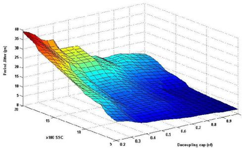
Fig.4. Output jitter dependence on average switching current and supply decoupling capacitance
